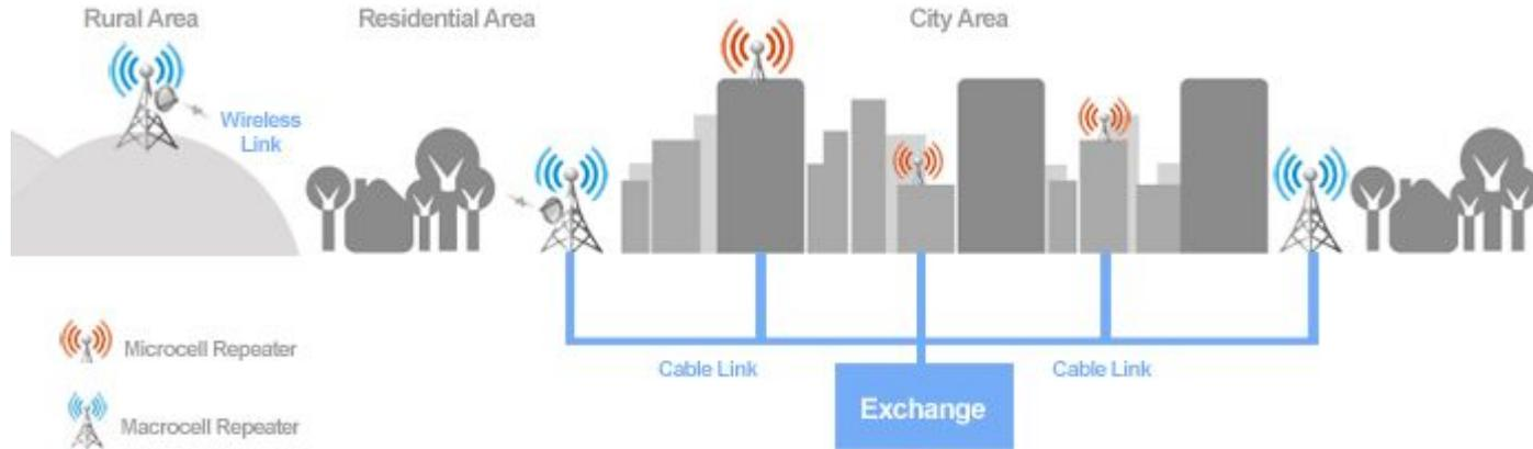
The cell coverage area is determined by the base station output power and the environment. Things such as trees, hills, buildings and land formations will have an effect on the coverage area.
